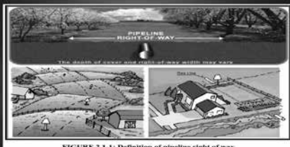
FIGURE 2.1-1: Definition of pipeline right of way
